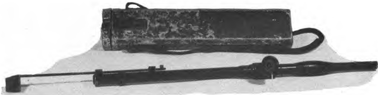
Figure 285. The hand held periscope, weighing 2.3 pounds, has a 5\times magnification and 10^\circ field of view.
