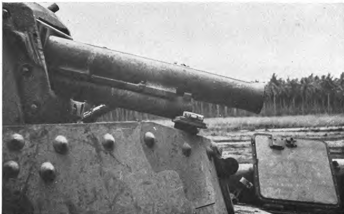
Figure 257. Model 97 (1937) 57-mm tank gun (showing its appearance from the outside of the turret).
