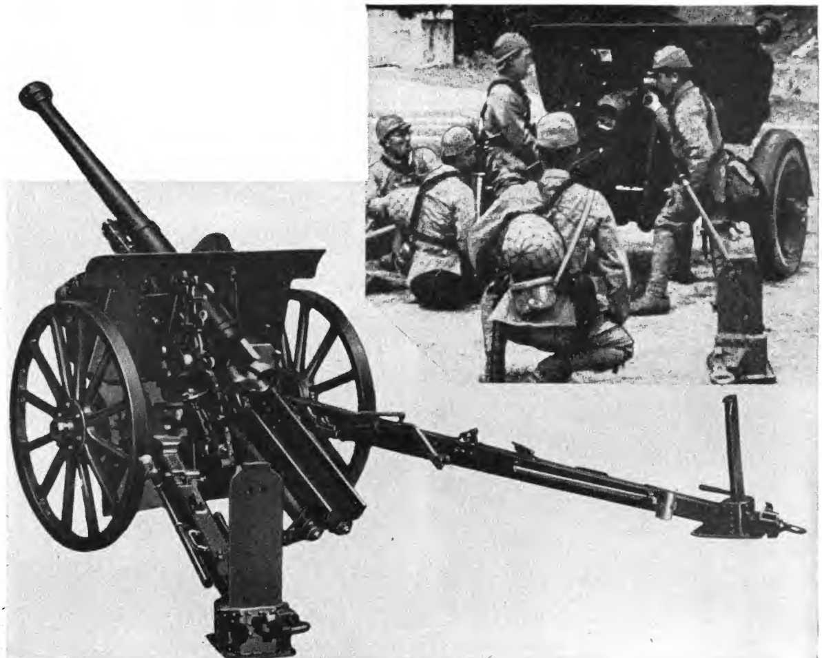
Figure 219. Model 90 (1930) 75-mm gun (inset shows the weapon on a high-speed carriage with pneumatic type tires).
