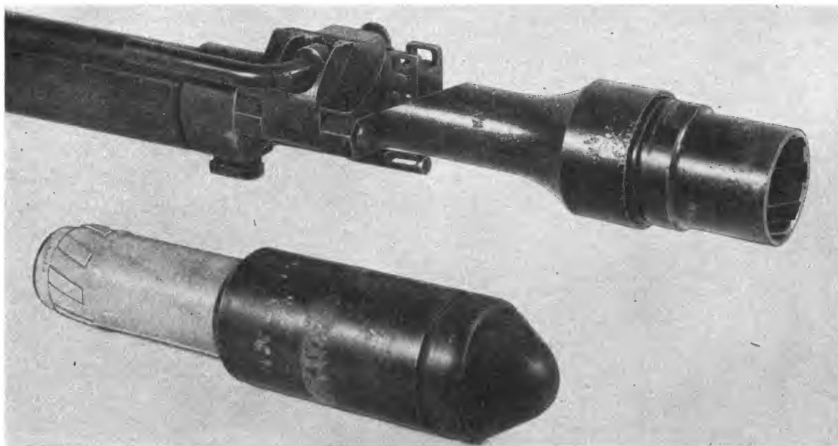
Figure 176. Rifled-type grenade launcher with armor piercing (hollow charge) rifle grenade.
