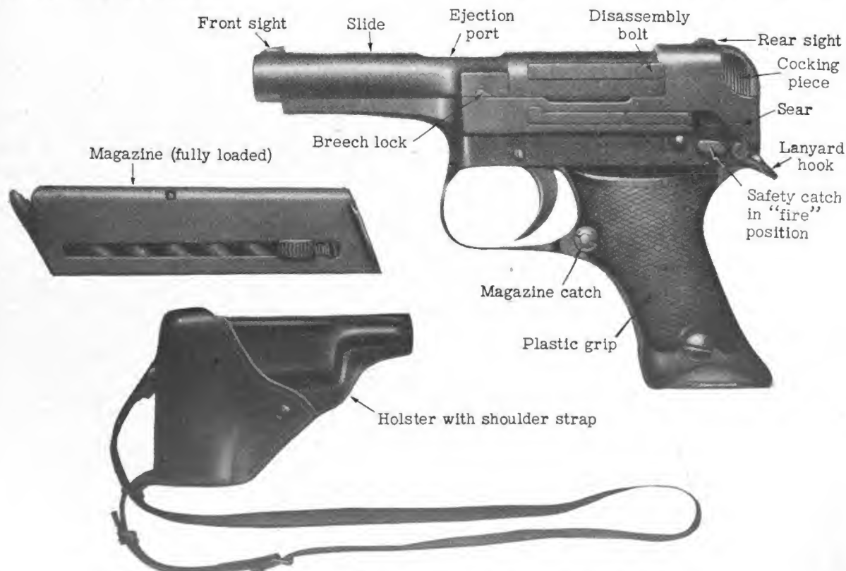
Figure 169. Model 94 (1934) 8-mm pistol, showing holster and magazine.
