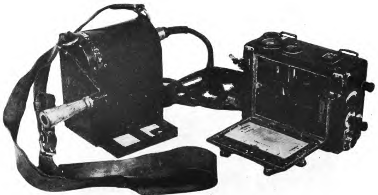
Figure 348. Model 97 Type 3. Transceiver, with hand generator. Pack type. Dipole elements of antenna fasten to wing nuts at ends of case.
