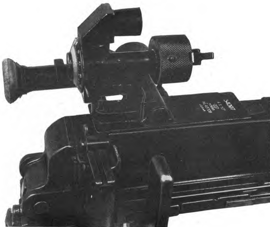
(Above) Figure 290. Telescopic sight for model 92 (1932) 7.7-mm machine gun has a 4\times magnification, a 10^\circ field of view, and a weight of 3 lbs., 6 ozs.
