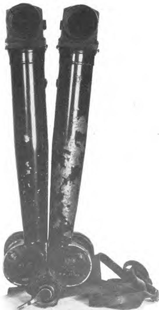
Figure 299. This battery commander's telescope has an 8\times magnification and a 6^\circ field of view. It is constructed so that the telescopic arms may be placed in a horizontal position for better stereoscopic vision.
