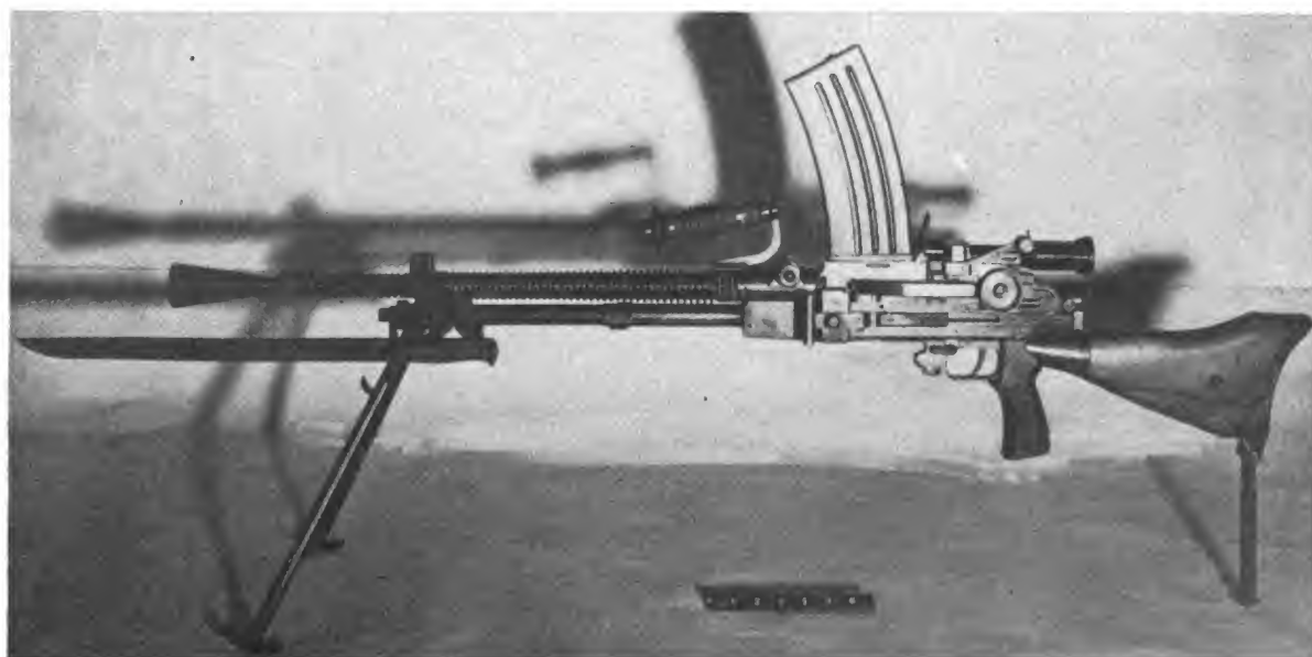
Figure 180. Model 99 (1939) 7.7-mm light machine gun.
