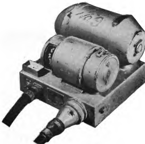
Figure 357. Dynamotor power supply for transmitter of model 96 Type 3 airborne radio set. Used in Type 1 medium bomber (Betty).
