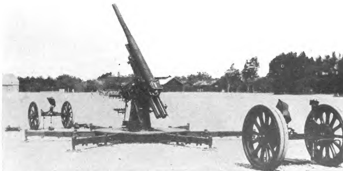
Figure 235. Model 14 (1925) 105-mm antiaircraft gun showing detachable wheels used for transport of piece.
