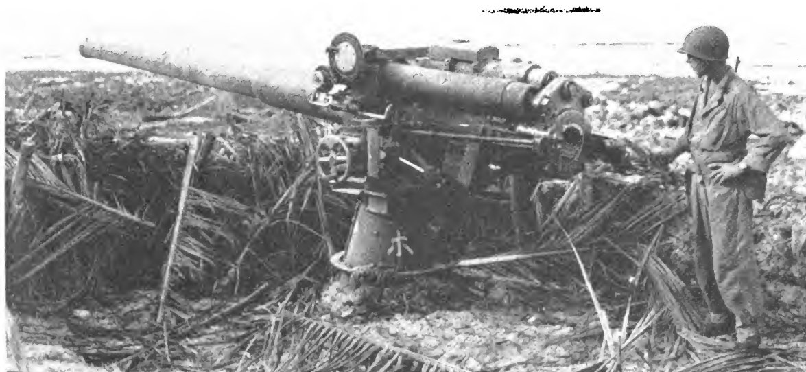
Figure 237. Model 3 (1914) 12-cm naval gun.
