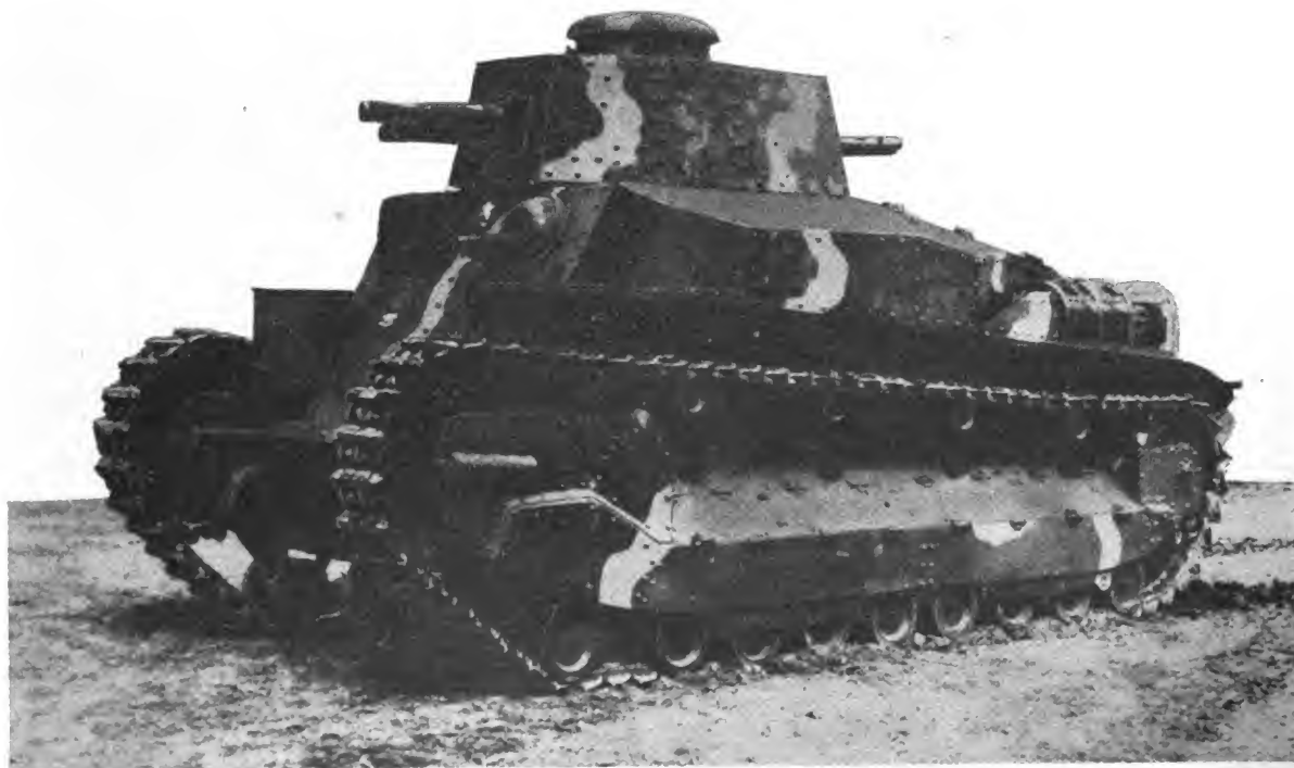
Figure 247. Model 94 (1934) medium tank.
