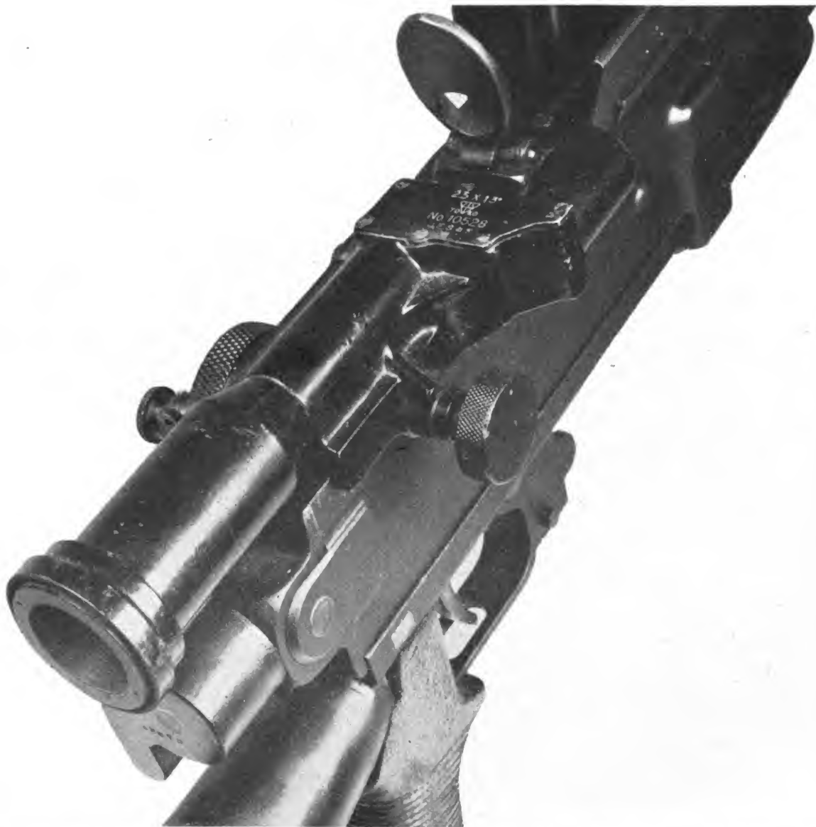
Figure 289. Telescopic sight for model 96 (1936) 6.5-mm light machine gun. The magnification is 2.5\times , the field of view is 13^\circ , and the weight is 20 oz. The reticle (Graticule) pattern provides for drift and windage, and is calibrated for a maximum range of 1,500 meters (1,640 yards).
