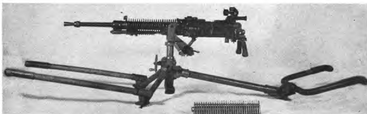
Figure 182. Model 92 (1932) 7.7-mm heavy machine gun—showing carrying handles and ammunition strip.
