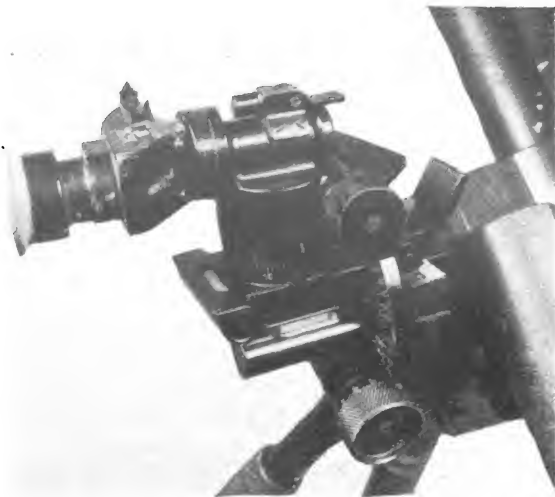
Figure 288. Panoramic sight for model 94 (1934) mortar has a 3\times magnification and a 13^\circ field of view. Micrometer drums enable readings to be made to the nearest mil.
