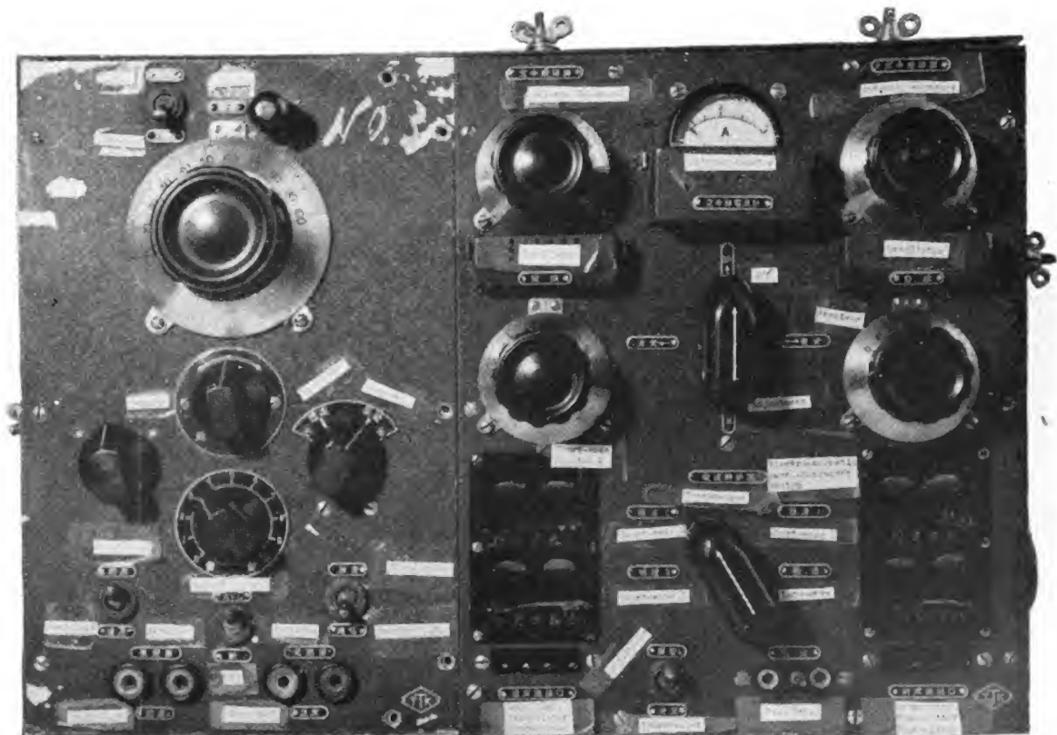
Figure 361. Model 96 (1936) Type 1. Transmitter-receiver model 13. From Mitsubishi bomber. Transmitter: 7600-10600 KC. Receiver: 7500-10800 KC.
