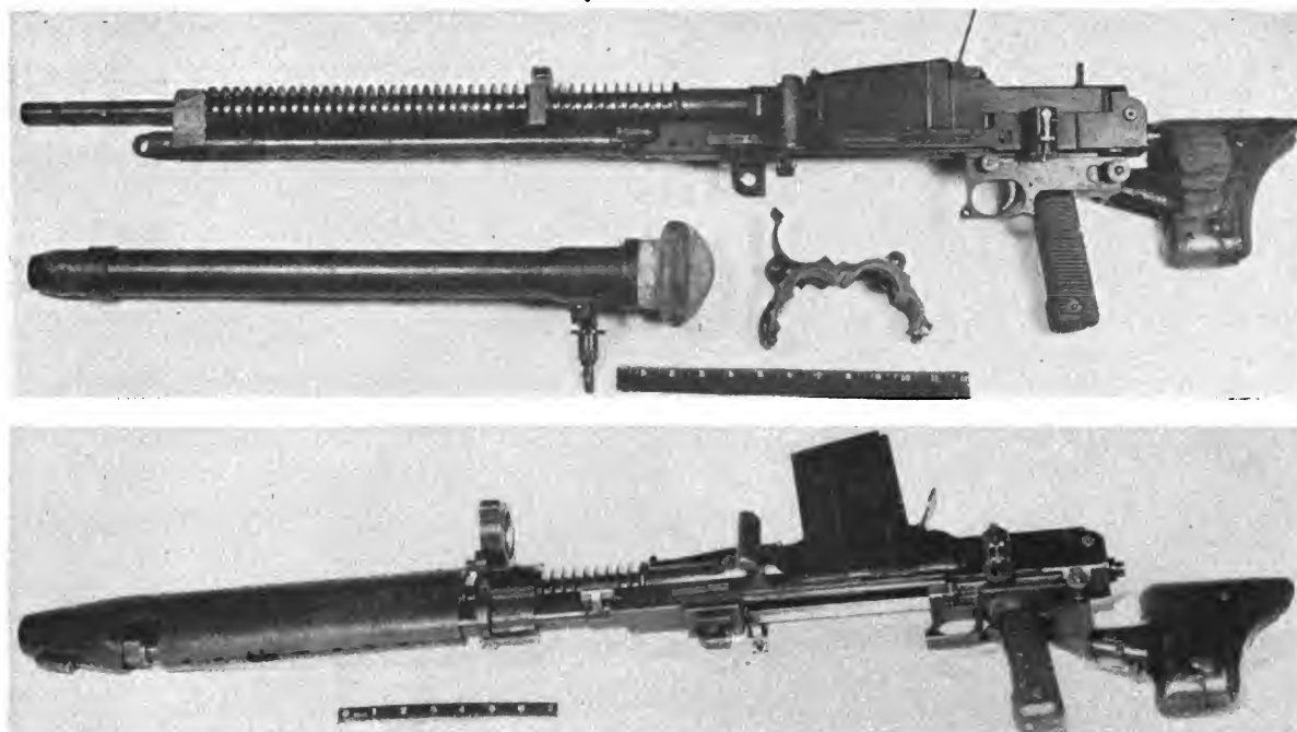
Figure 255. Model 97 (1937) 7.7-mm tank machine gun. (The lower figure illustrates the armor shield normally used when this machine gun is mounted in a tank.)
