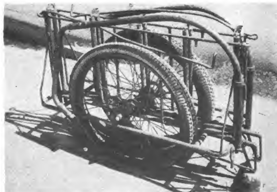
Figure 405. Collapsible hand cart of metal construction weighing 100 pounds. It may be pulled by hand or towed by bicycle.
