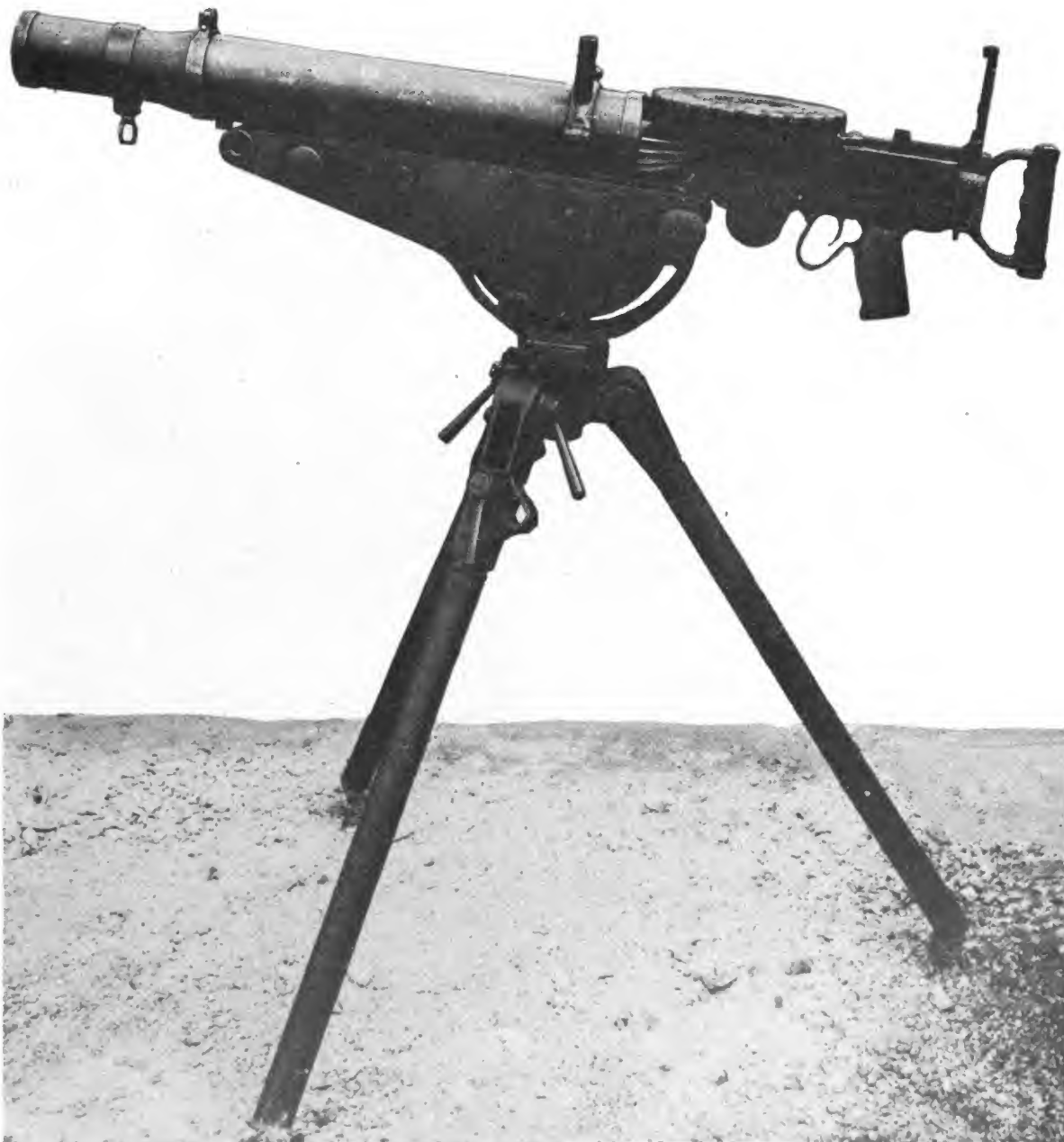
Figure 181. Model 92 (1932) 7.7-mm Lewis type machine gun.
