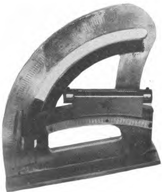
Figure 304. This gunner's quadrant is calibrated from 0 to 90^\circ , with a vernier reading to \frac{1}{16} of a degree.
