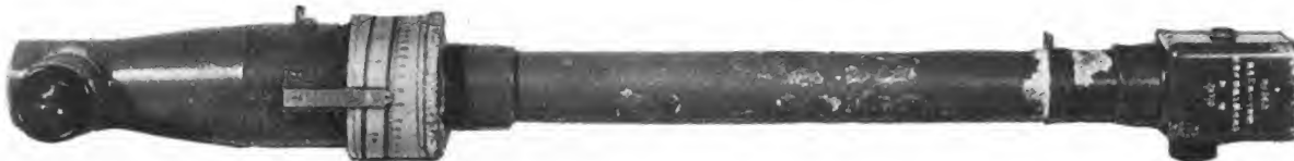
Figure 286. Model 92 (1932) 40-cm base range finder is calibrated for measuring ranges up to 1,500 meters (1,640 yards). It is a coincidence type of range finder with a 4\times magnification.
